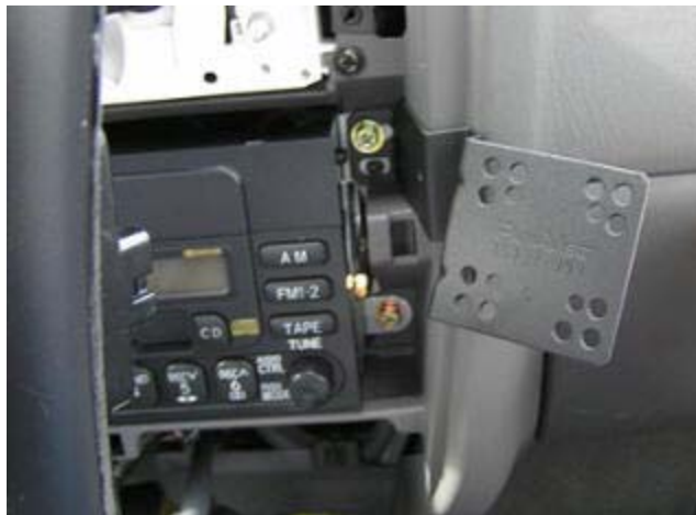
InDash mounted showing screw location
